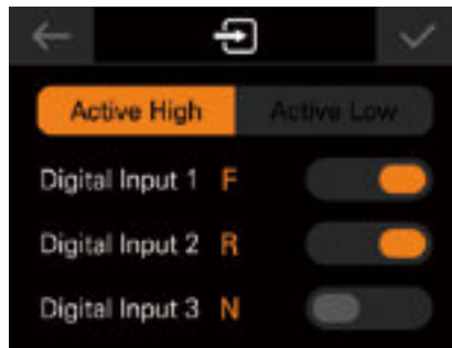
⑧ Active value and activate Input signal · F : Forward (Applies forward detection range) · R : Reverse (Applies backward detection range) · N : Neutral (Alarm cancel state)
