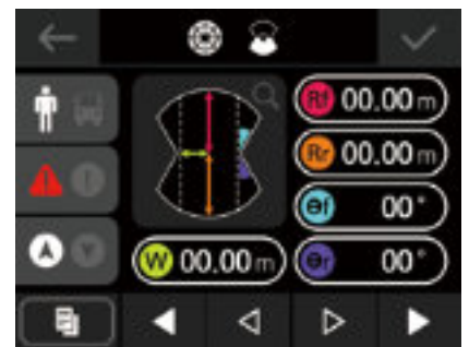
⑥ Set Warning/Danger zone by entering distance & angle (front/rear, left/right) from the reference point 📄 Copy value
